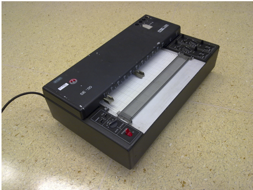
Figure 4.1: A simple two channel x,t-recorder. Two pens are pressed against the paper which is fed through underneath the pens.
